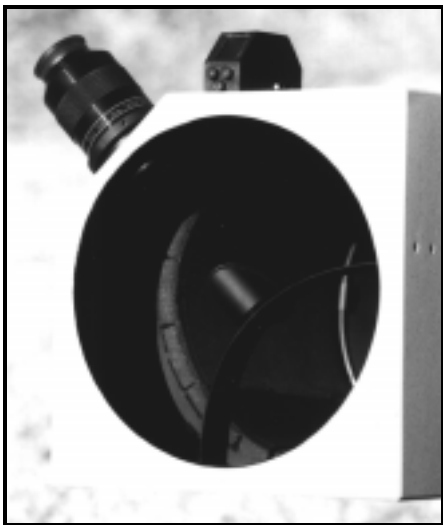
Spider, diagonal holder, and shroud
