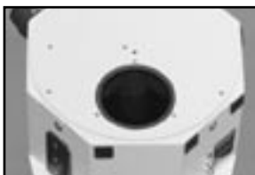
Fig. 31: Mask used to reduce aperture
