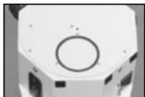
Fig. 30: Mask with cover plate to block dust
