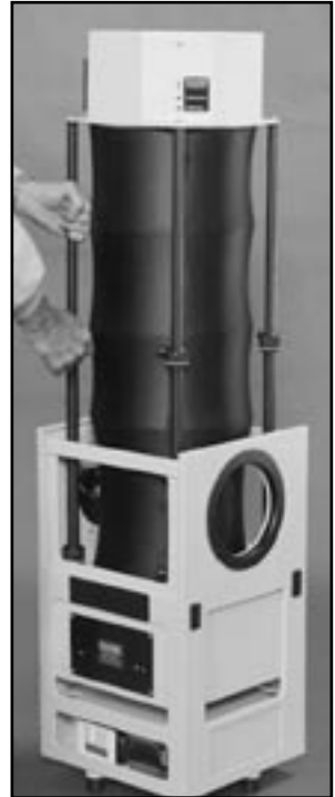
Fig. 15: Tighten both clamps on each strut
