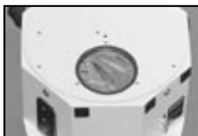
Fig. 32: Mask with solar filter in place
