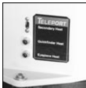
Fig. 26: Secondary cage outlets and heater switch
