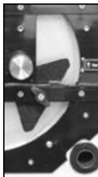
Fig. 25: Fan switch on primary mirror cell
