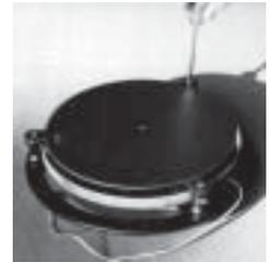
Fig 10: Remove the mirror lock plate
