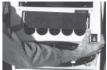
Fig 43: Opening the airknife exhaust cover
