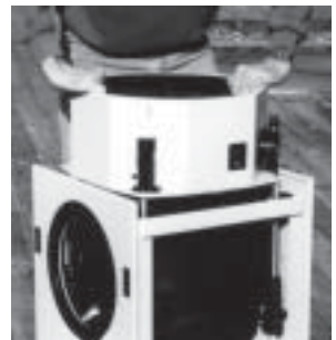
Fig 19: Grasp the secondary cage
