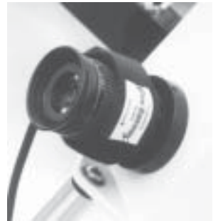
Fig 27: heating the eyepiece
